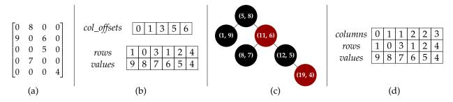
**Figure 2:** Illustration of sparse matrix representations: (a) example sparse matrix with 5 rows, 4 columns and 6 non-zero values, shown in traditional mathematical notation; (b) corresponding CSC representation; (c) corresponding RBT representation, where each node is expressed by (i, v), with *i* indicating a linearly encoded matrix location and *v* indicating the value held at that location; (d) corresponding COO representation. Following C++ convention [31], we use zero-based indexing.
